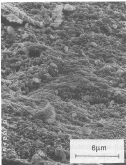
Fig. 14. Fracture surface of hot-pressed HDDR magnet revealing uniform fine-grain size.
